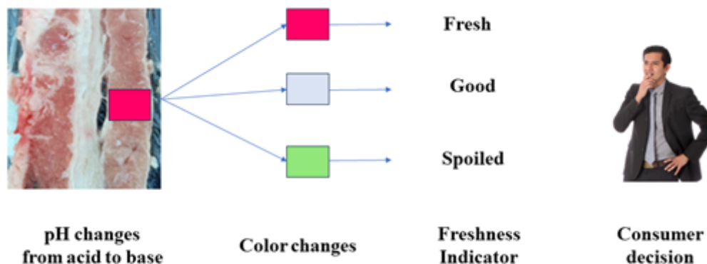
Figure 8. Schematic of the Developed Freshness Sensor Mechanism
