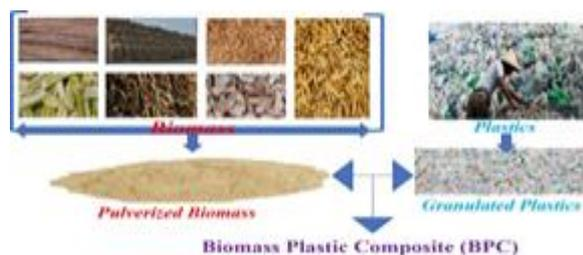
**Figure 1. Illustration of Biomass Plastic Composite (BPC) Fabrication**
