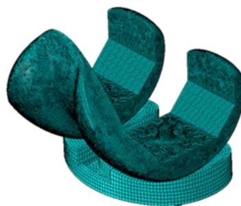
Figure 3. 3D FE Model of the BCR-TKA Implant
