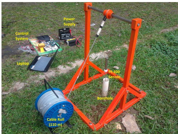
Figure 9. The Prototype of Temperature Logging Tools
