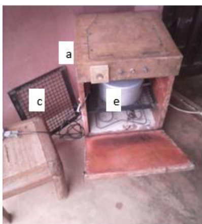
Figure 2. Covered Stockpot with Water and the Remote Thermometer Inside the Oven for Testing Operation: (a) Oven, (c) Meshed Tray, (e) Stockpot with 6 Litres of Water Inside the Oven
