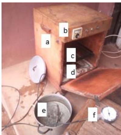
Figure 1. Fabricated Conventional Electric Oven and the Test Apparatus: (a) Oven, (b) Controls, (c) Mesh Tray, (d) Heating Element, (e) Stockpot with Water and Remote Thermometer Sensor Inside, (f) Remote Thermometer
