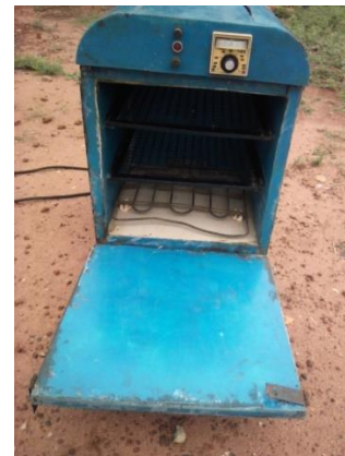
Figure 3. Interior of the Chamber of the Electric Oven
