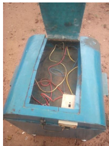
Figure 4. Electrical Wiring Compartment of the Oven
