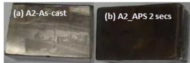
Figure 1. Samples of (a) A2 ASS as-cast and (b) A2 ASS after APS for 2 s
