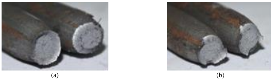
Figure 4. Type of Fracture Observed on the Sample BJTP24 Ø10 mm: Nearly Cup-and-Cone
