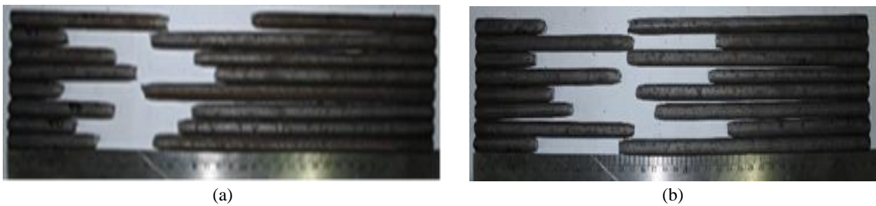
Figure 3. Fracture Location of BJTP24 Ø10: (a) Side A and (b) Side B
