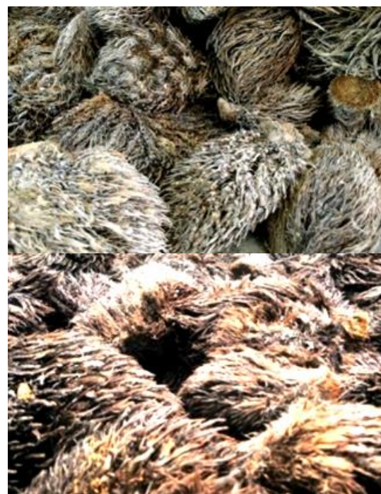
Figure 1. EFB Waste as the Basic Material for Making Bio-Briquettes
