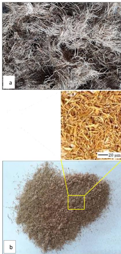
Figure 2. EFB : (a). Fiber Before Chopping; (b). Fiber After Being Chopped and Filtered on a 20 Mesh
