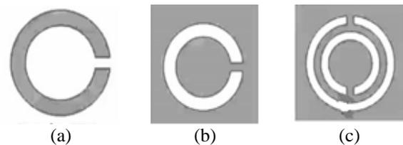
**Figure 4. (a) Circular Split-ring Resonator, (b) Circular Complementary Split-ring Resonator, and (c) Double Circular Split-ring Resonator**
