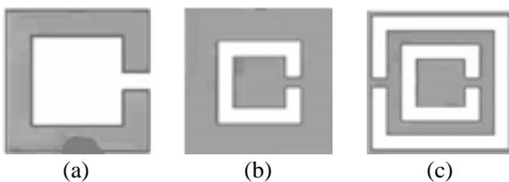
**Figure 3. (a) Square Split-ring Resonator, (b) Square Complementary Split-ring Resonator, and (c) Double**
