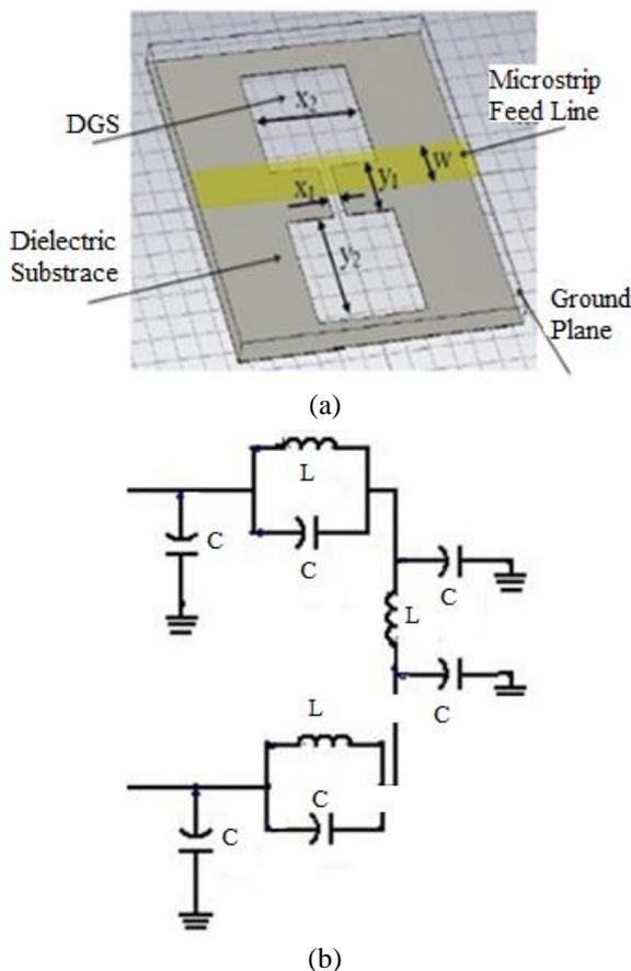
**Figure 1.** (a) Layout of Dumbbell-DGS Unit in Ground Plane of Substrate, and (b) Equivalent Model of Dumbbell-DGS Unit
