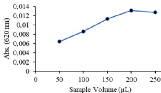
Figure 11. Effect of Sample Volume on Extract Absorbance (620 nm)
