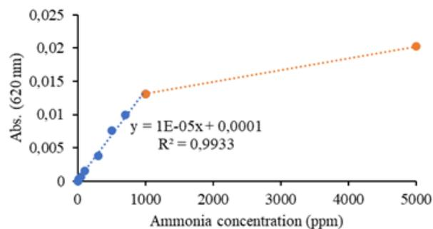
Figure 12. Ammonia Concentration Relationship Curve with Absorbance in the Linearity Test
