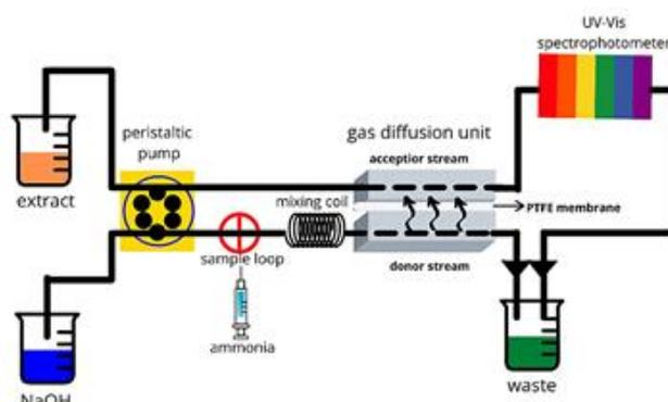
Figure 4. GD-FIA spectrophotometry manifold
