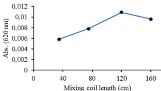
Figure 10. Effect of Mixing Coil Length on Extract Absorbance (620 nm)
