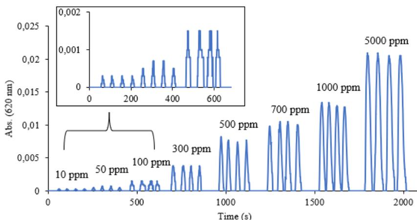
Figure 13. FIA-gram Profile of Standard Ammonia at 10–5000 ppm for the Calibration Curve
