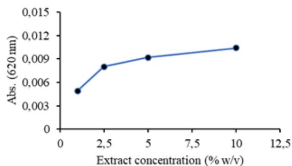
Figure 9. Effect of Extract Concentration on Absorbance at 620 nm
