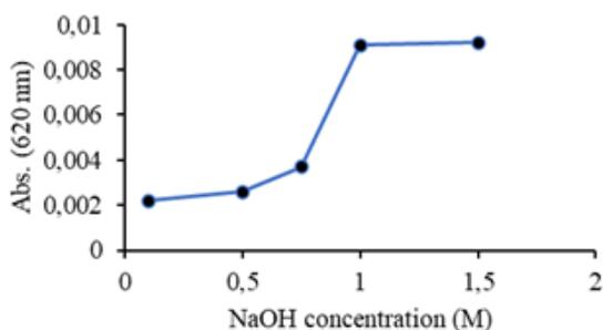
Figure 8. Effect of NaOH Concentration on Extract Absorbance (620 nm)
