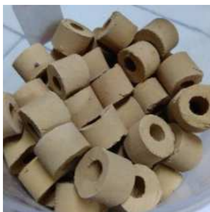
Figure 1. a. Apparatus for Ethanol Purification; b. Zeolite Packing
