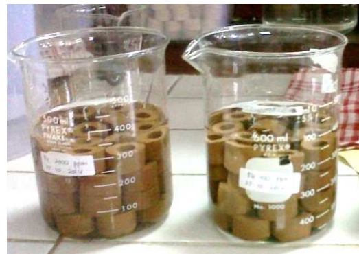
Figure 1. Zeolite/bentonite Rings under Cation Exchange
