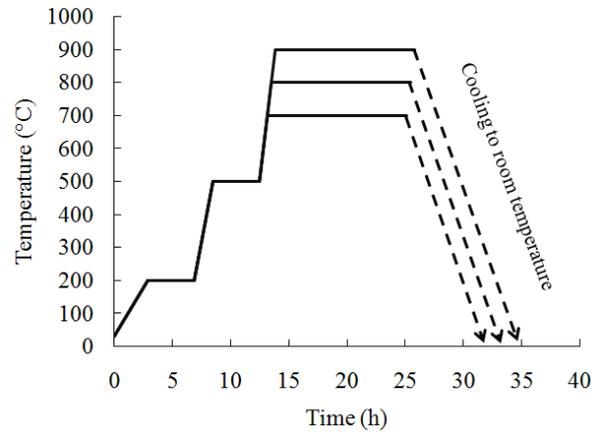
**Figure 2. Heat Treatment Programs of the Composite Samples over a Range of Sintering Temperatures**
