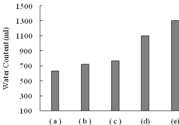
**Figure 1. Water Content (ml) Required by Each Composite:** (a) Clay/Iron Sand (b) Clay/Iron Sand/RHA1 (c) Clay/Iron Sand/RHA2 (d) Clay/RHA1 and (e) Clay/RHA2
