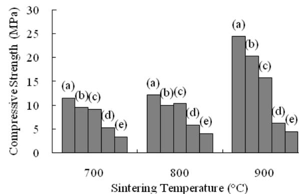
**Figure 3. Compressive Strength of the HTC: (a) Clay/iron sand (b) Clay/iron sand/RHA1 (c) Clay/iron sand/RHA2 (d) Clay/RHA1 and (e) Clay/RHA2 Over a Range of Sintering Temperatures**
