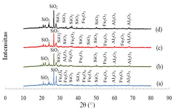
**Figure 4. The XRD Diffraction Pattern of Heat-treated Composite at Sintering Temperature of 900 °C for: (a) Clay/Iron Sand, (b) Clay/Iron Sand/RHA1, (c) Clay/Iron Sand/RHA2 and (d) Clay/RHA2**
