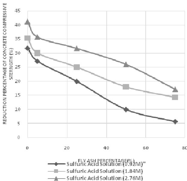
Figure 2. Relation of Fly Ash Utilization towards Reduction Percentage in Concrete Compressive Strength for H<sub>2</sub>SO<sub>4</sub> Solution as Immersion Media
