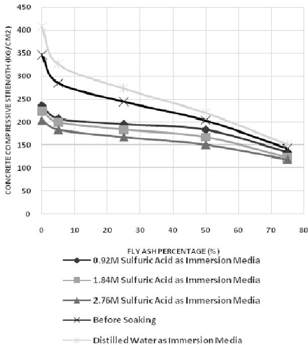
**Figure 1. Relation of Fly Ash Replenishment in Concrete towards Concrete’s Compressive Strength in Varied Immersion Media**
