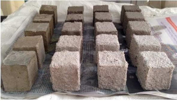
**Figure 4. Appearance of Concrete Samples after Immersion Process**
