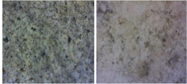
**Figure 5. Structures of Morphology of Concrete Surface (Magnification 35x) Soaked in Distilled Water (Left) and in 2.76M Sulfuric Acid Solution (Right)**
