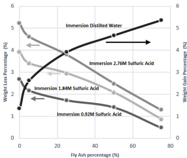
**Figure 3. Relation of Fly Ash Replenishment in Concrete towards Concrete's Weight Change Percentage in Varied Immersion Media**
