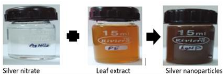
Figure 2. Pictorial Representation of the Synthesis of the Nanomaterials Showing the Colors of the Reactants and the Product [2]
