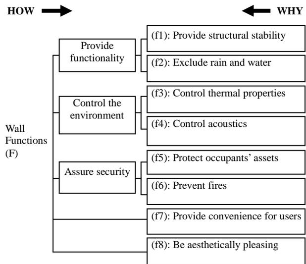
**Figure 2. The FAST Diagram of the Wall System**
