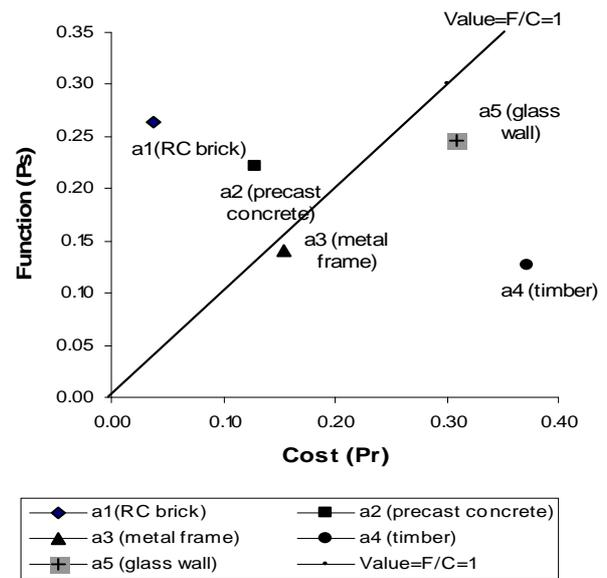
**Figure 4. Basic Values of Wall System Options**
