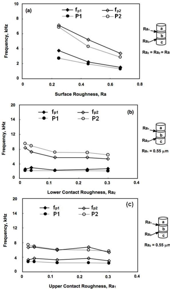
**Figure 9.** Effect of Contact Stiffness on Peak Frequencies; Similar Roughness for Upper and Lower Contact Interfaces (a), Different Roughness for Lower Contact Interface (b), and Different Roughness for Upper Contact Interface (c)
