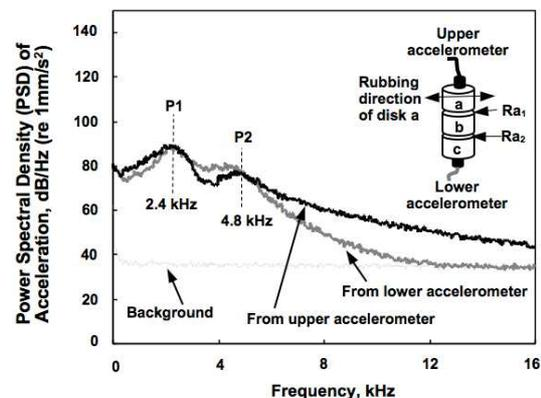
Figure 2. Comparison between Power Spectral Density (PSD) of Acceleration Obtained from Upper and Lower Accelerometers and that of Background Acceleration
