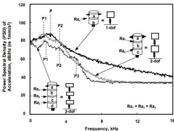
Figure 7. Dynamic Modeling of Disks in Configuration and Occurrence of Peaks at Frequency Response Functions; all Contact Interfaces have Similar Roughness
