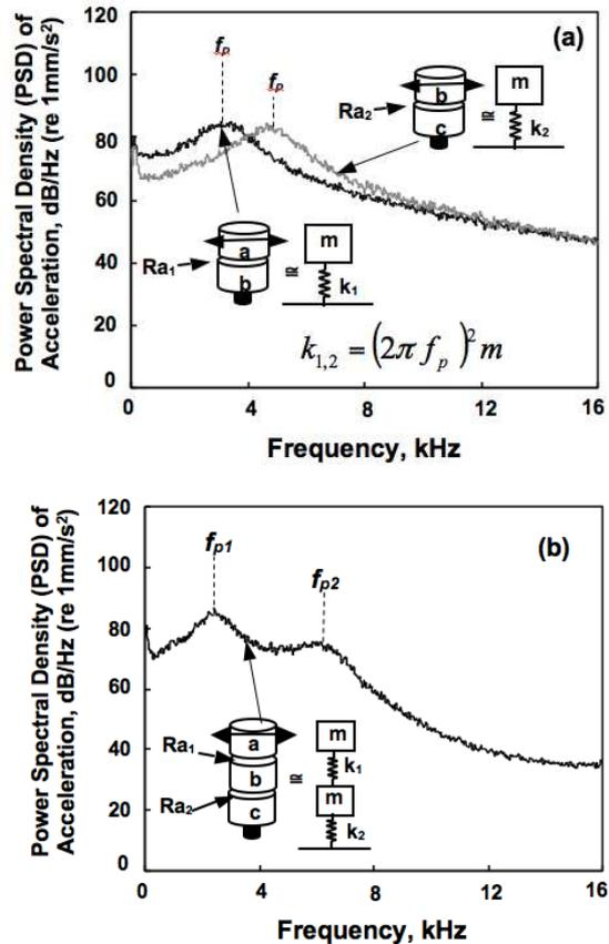
Figure 8. A Method for the Estimation of Peak Frequencies; Peak Frequencies Obtained from Rubbing the Two-disk Configuration are Used to Calculate the Contact Stiffness of the Respective Contact Combinations (a). The Values of Contact Stiffness are Used in the 3-disk Configuration Model (b) to Estimate the Peak Frequencies  $f_{p1}$  and  $f_{p2}$  using Equation 1
