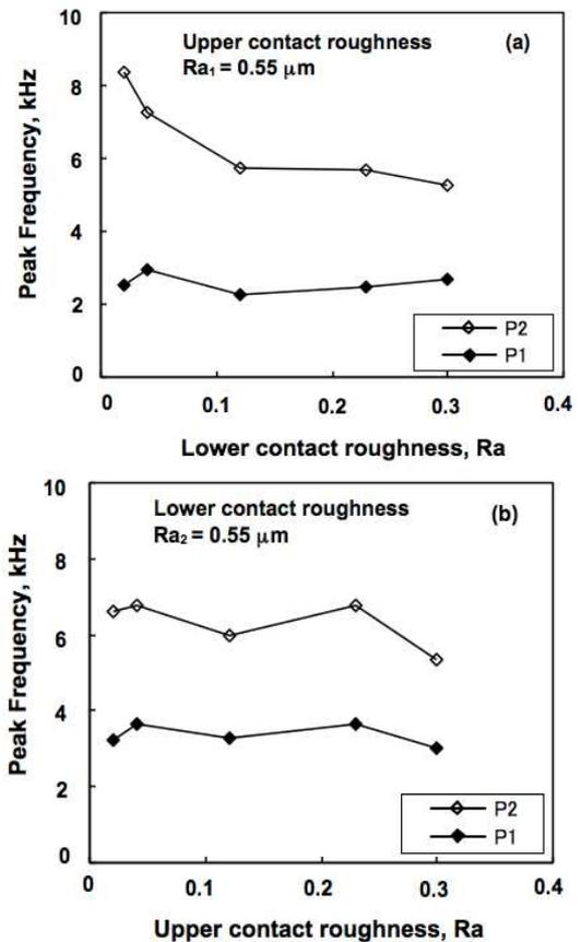
**Figure 5. Effect of Roughness on Peak Frequency Shift in the 3-disk Configuration for Test Condition A (a), and Effect of Roughness on Peak Frequency Shift of 3-disk Configuration for Test Condition B (b)**
