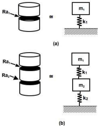
Figure 6. Dynamic Model of Disks in Contact
