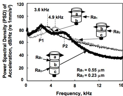
**Figure 4. Rubbing of 3-disk Configurations with Different Levels of Roughness at the Upper and Lower Contact Interfaces; Comparison between Power Spectral Density (PSD) Obtained from 2-disk Configuration and from 3-disk Configuration**
