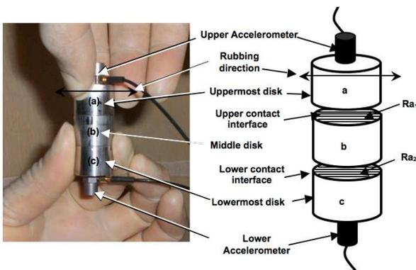
Figure 1. Three-disk Configuration Rubbing by Hand
