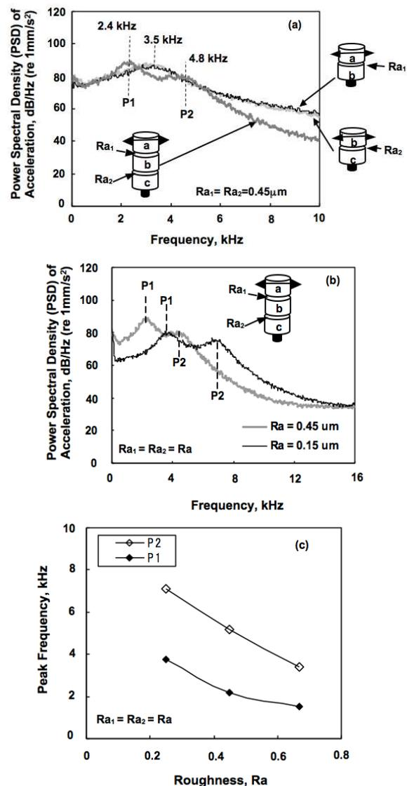
**Figure 3. Rubbing of 3-disk Configurations with Similar Roughness at Both Upper and Lower Contact Interfaces; Comparison between Power Spectral Density (PSD) obtained from 2-disk Configuration and that from 3-disk Configuration (a), Effect of Roughness on PSD of 3-disk Configuration (b), and Effect of Roughness on Peak Frequency Shift of 3-disk Configuration (c)**
