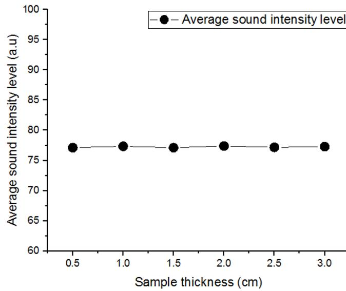
Figure 8. Ratio of the Thickness of the Sample to the Level of the Average Sound Intensity Produced
