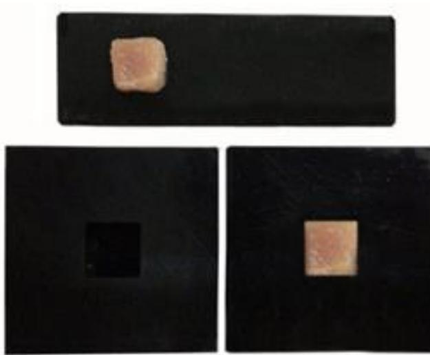
**Figure 2.** Acrylic Box (Below) as the Control of Sample Dimensions and Thickness and Black Glass (Above) as the Sample base in Imaging
