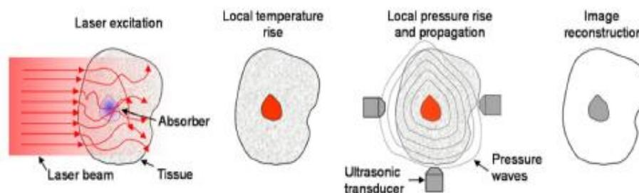
Figure 1. PAT Imaging Principle [6]
