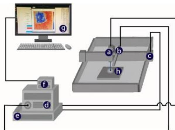
**Figure 3.** Schematic of the Photoacoustic Tomography Imaging System based on (a) Diode Laser, (b) Electret Condenser Microphones, (c) Motor Stepper, (d) Soundcard, (e) Microcontroller, (f) Raspberry Pi, (g) Interface Screen, and (h) Sample/Object [9]
