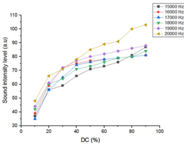
Figure 5. Plot of Frequency and Duty Cycle Data against the Level of Sound Intensity Produced
