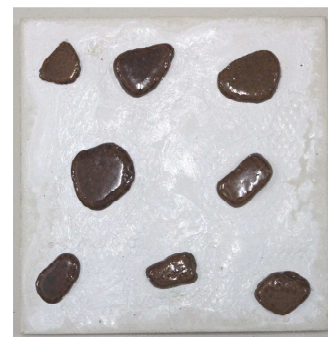
Figure 2. Type I; Tile Body Made of White Portland Cement, Surface Topping with Artificial Pebbles
