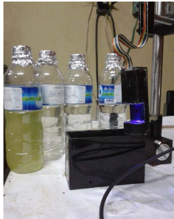
Figure 2. Optical Probe and Measurement Container
