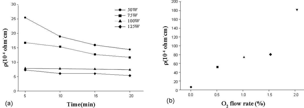
Figure 5. Resistivity of ITO Films Varied with (a) Deposition Time and RF Power, and (b) Oxygen Admixture
