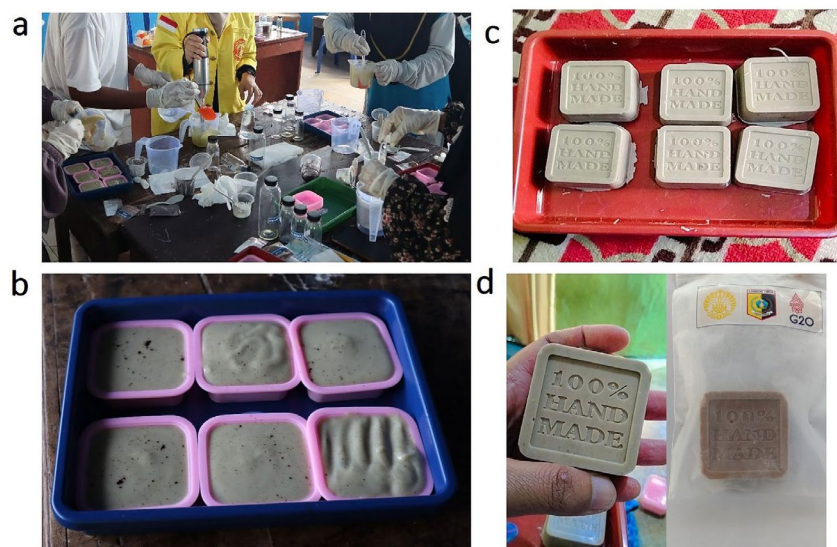
Figure 3. The activity documentation: a) soap making workshop; b) soap before drying process; c) soap after three-day drying process; and d) ready-to-use soap after 1 month
