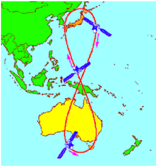
Figure 1. Quasi-Zenith Satellite Orbit [1]
