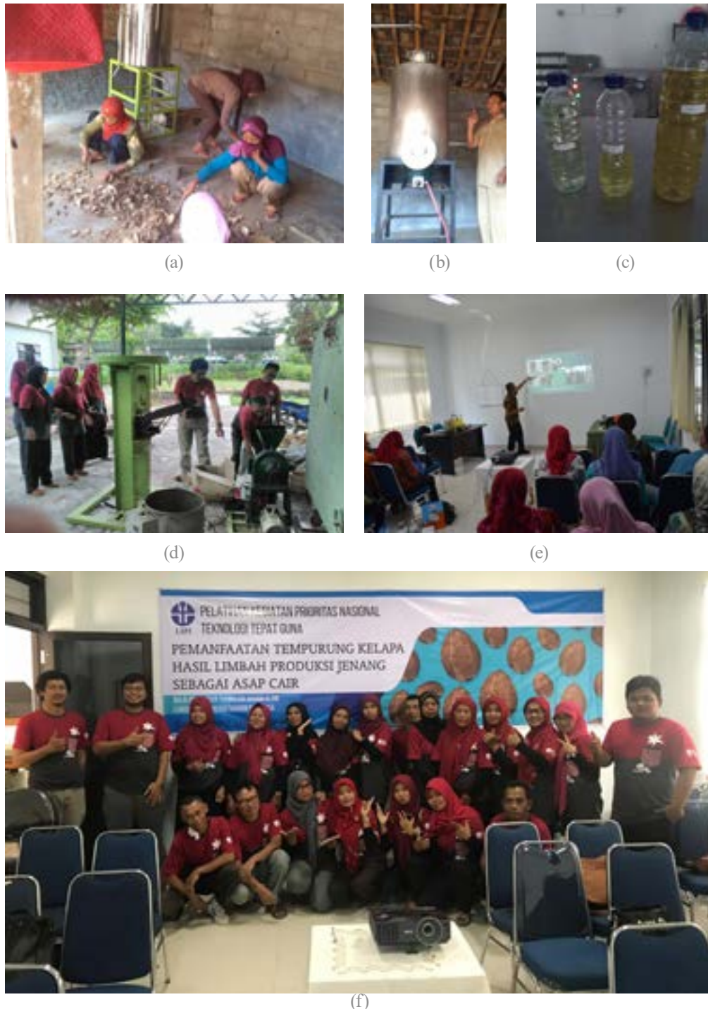
Figure 5. Documentation of training and workshop activities for processing coconut shell waste into liquid smoke and bio-briquette: (a) preparation of drying coconut shell waste, (b) practicing pyrolysis of dried coconut shell waste, (c) liquid smoke obtained from left to right (crude and after distillation), (d) charcoal grinding process, (e) theoretical class, and (f) participants in the training and workshop
