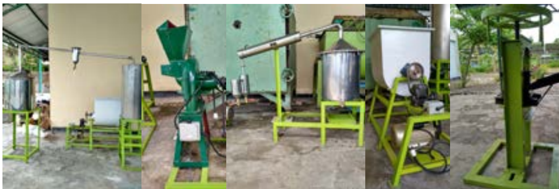
(a) (b) (c) (d) (e) Figure 4. The instruments procured for coconut shell waste processing into liquid smoke and bio-briquette in Bohol Village: (a) pyrolysis reactor, (b) grinder machine distillation, (c) reactor, (d) mixer machine; (e) briquette press machine
