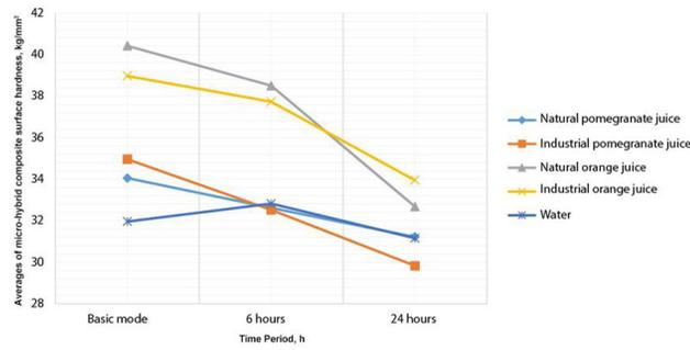
Figure 1. Averages of micro-hybrid composite surface hardness in 3 time periods for each beverage group
