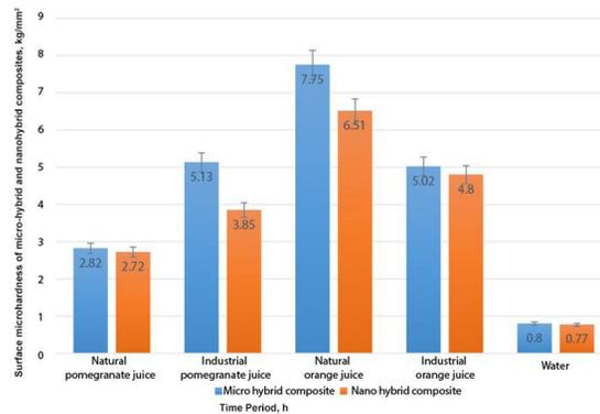
Figure 3. Comparison of the effect of natural and industrial juices on the surface microhardness of micro-hybrid and nano-hybrid composites
