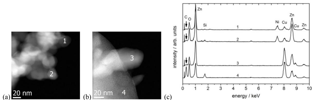
**Figure 5.** STEM-HAADF Images of (a) Fresh and (b) Used ZnO/(60)SiO<sub>2</sub> Catalysts and (c) the Corresponding EDX Analysis
