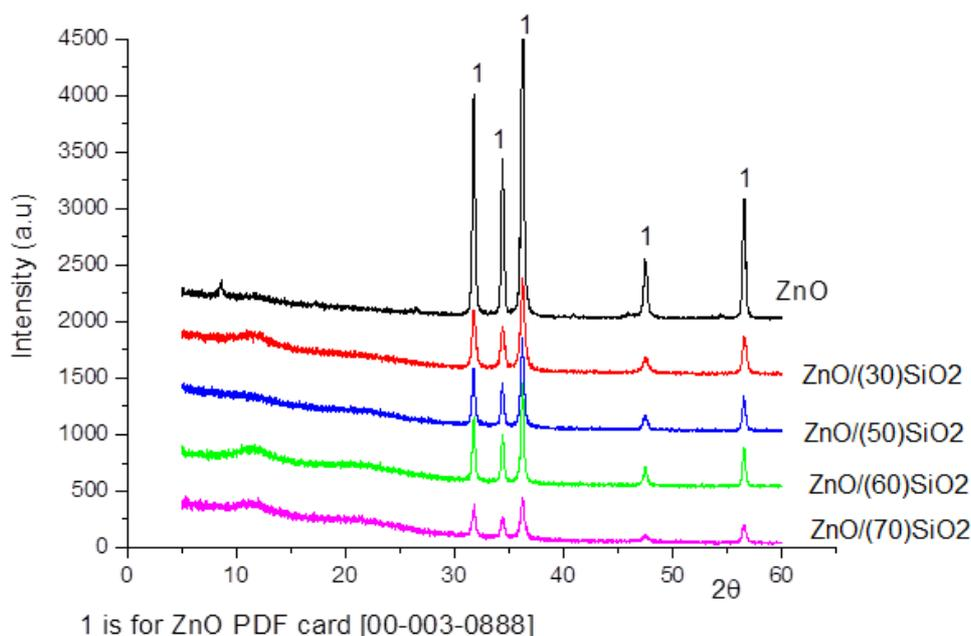
Figure 2. XRD Patterns of  $\text{ZnO}/(x \text{ wt}\%)\text{SiO}_2$  Catalysts and ZnO Standard
