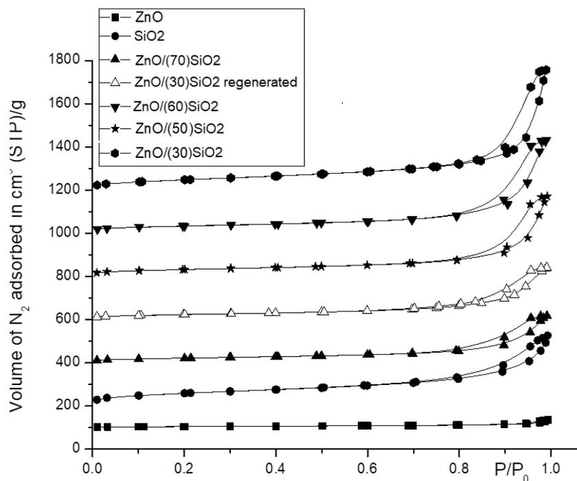
**Figure 3. Adsorption–desorption Isotherms of the ZnO/(x)SiO<sub>2</sub> Composites**
