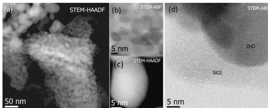
**Figure 4.** STEM Images of the Fresh ZnO/(60)SiO<sub>2</sub> Catalyst. (a) Dark-field Image of the Two Particle Sizes, (b) Bright-field Image of ZnO Crystals of 5–10 nm, (c) Dark-field Image of ZnO Crystals of 20–50 nm, and (d) Bright-field Image of ZnO Crystals and Silica
