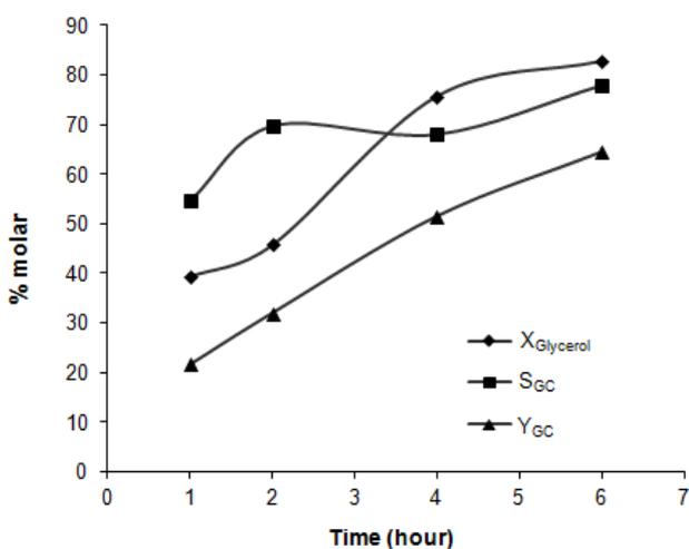
**Figure 8.** Results of the Reaction between Glycerol and Urea in the Presence of ZnO/(60)SiO<sub>2</sub> as a Function of Reaction Time. Reaction Conditions: Glycerol/Urea Molar Ratio = 1:1,  $P = 30$  mbar,  $T = 140$  °C
