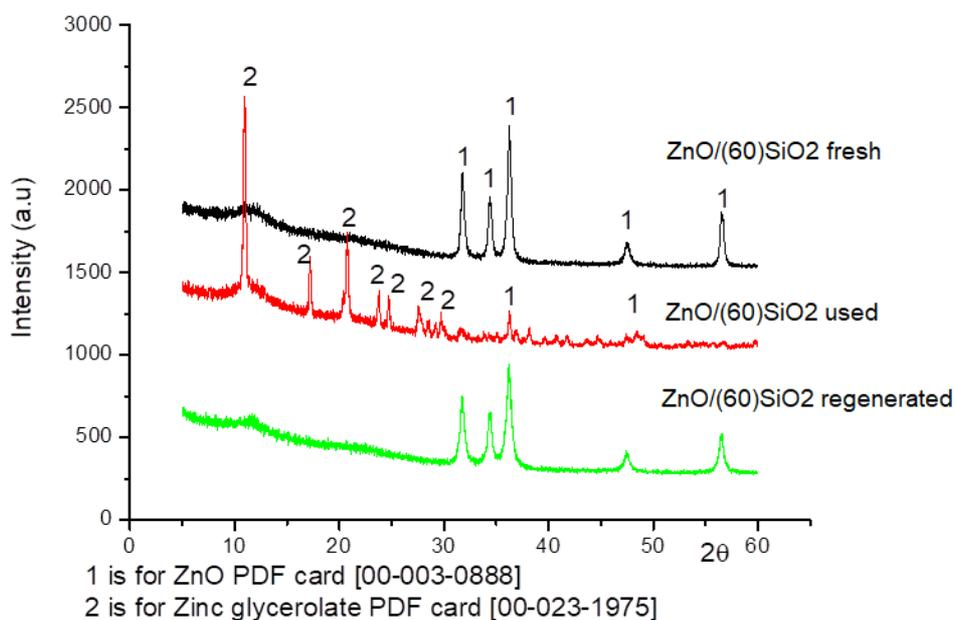
Figure 10. XRD Patterns of ZnO/(60)SiO<sub>2</sub>
