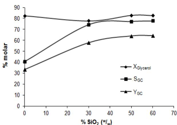
**Figure 7.** Results of the Reaction of Glycerol with Urea in the Presence of ZnO/(60)SiO<sub>2</sub> Catalyst as a Function of SiO<sub>2</sub> Content. Reaction Conditions: Glycerol/Urea Molar Ratio = 1:1,  $P = 30$  mbar,  $T = 140$  °C,  $t = 6$  h
