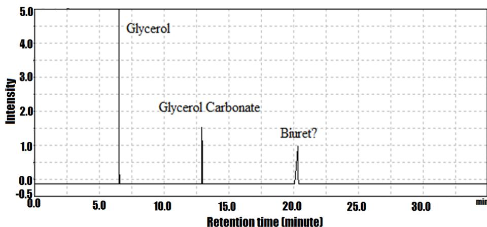
**Figure 6.** Chromatogram of Products from the Reaction between Glycerol and Urea Using ZnO/(40)SiO<sub>2</sub> Catalyst. Reaction Conditions: Glycerol/Urea Molar Ratio = 1:1,  $P = 30$  mbar,  $T = 140$  °C,  $t = 6$  h
