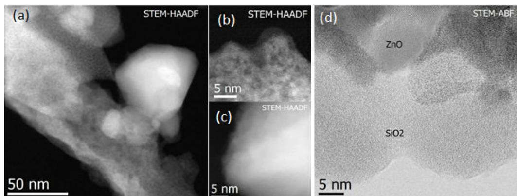
**Figure 11.** STEM Images of the Used ZnO/(30)SiO<sub>2</sub> Catalyst. (a) Dark-field Image as an Overview and (b) Dark-field Image with Higher Magnification of Small Particles (1–3 nm). (c) HAADF Image Showing a ZnO Cluster (Dark Gray) on the SiO<sub>2</sub> Crystal Surface (White). (d) ABF Image of the Silica and ZnO Crystals
