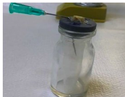
Figure 1. Installation of experimental device. An external glass bottle was used to stabilize the tooth and the residual recipient tube. A needle inserted into the bottle's silicone cap was used to equalize the pressure.
