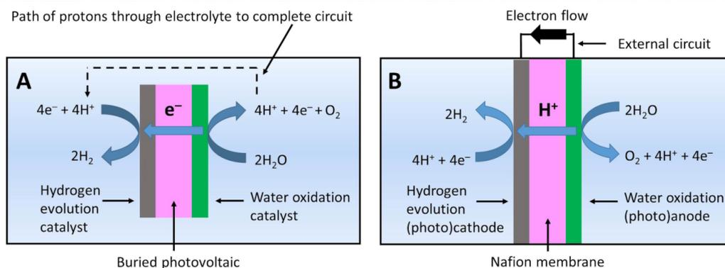
**Figure 1. Two Generic Representations of Artificial Leaves. A) A Wireless Configuration with no Separation of the Product Gases. B) A Wired Configuration in which the Electrical Circuit is Completed by External Wiring. In this Latter Conformation, one or both of the Electrodes will also Incorporate Light-harvesting Semiconductors, making a Photo-Catalytic Ensemble**
