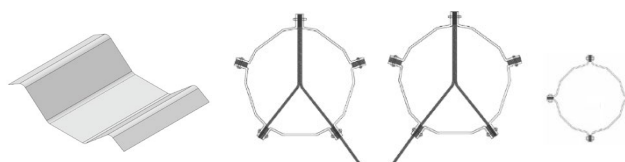
Figure 1 Illustration of individual plate and the proposed semi-closed polygonal cross section for chords and diagonals
