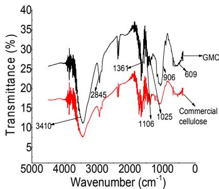
**Figure 1. Fourier Transform-Infrared Spectra of Commercial Cellulose and Golden Melon Skin (GMC)**
