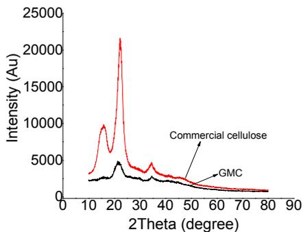
**Figure 2. X-ray Diffraction Spectra of Commercial Cellulose and Golden Melon Skin (GMC)**
