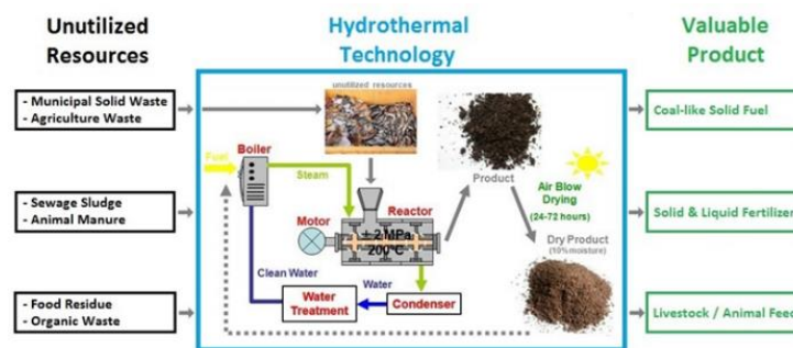
Figure 4 Hydrothermal technology process Source: Serpong Urban Residential’s Developer Concept
