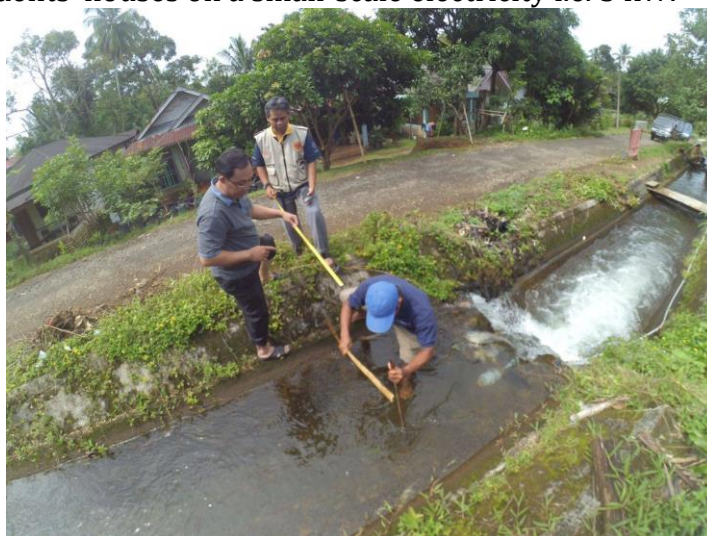
Fig. 2 Engineering team measure water discharge in Batu Roto's waterways Source: Dendy Adanta (2017)
