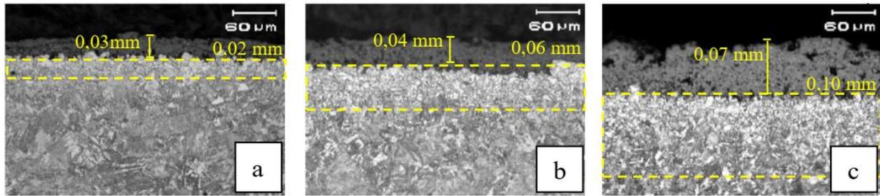
FIGURE 5. Microstructure Observation on the Surface Area. (a) Q1, (b) Q2, (c) Q3.
