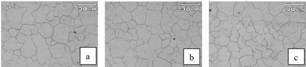
FIGURE 3. Prior Austenite Microstructure. (a) Q1, (b) Q2, (c) Q3.
