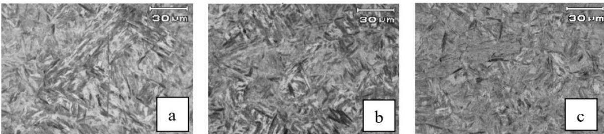
FIGURE 4. Martensite Microstructure. (a) Q1, (b) Q2, (c) Q3.
