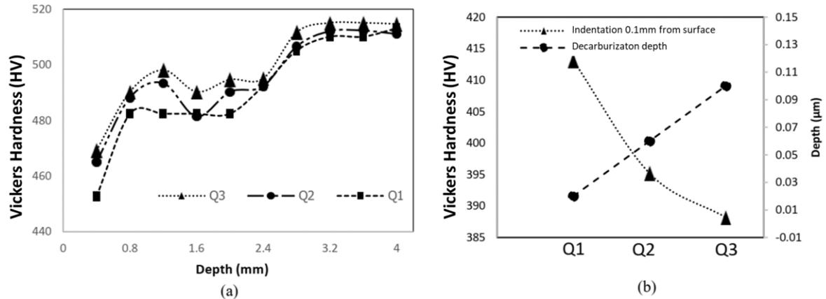
FIGURE 6. (a) Hardness in Different Surface Depth, (b) Hardness Value comparison with Decarburization Depth.
