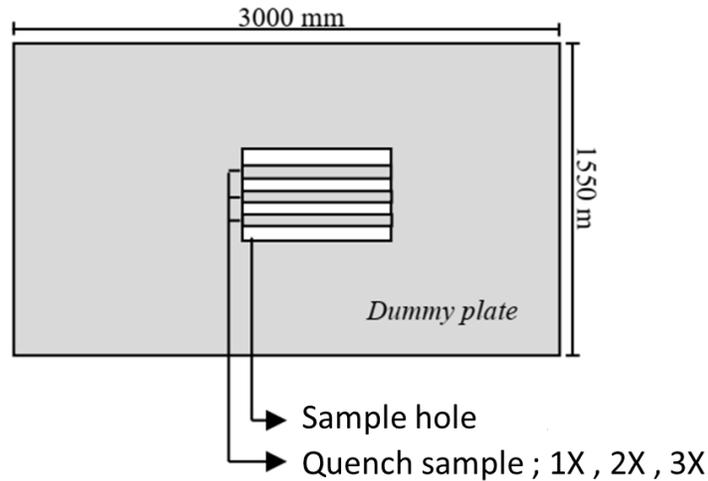
FIGURE 1. Sample Preparation Scheme on Heat Treatment Process in Rolled Quencher Facility
