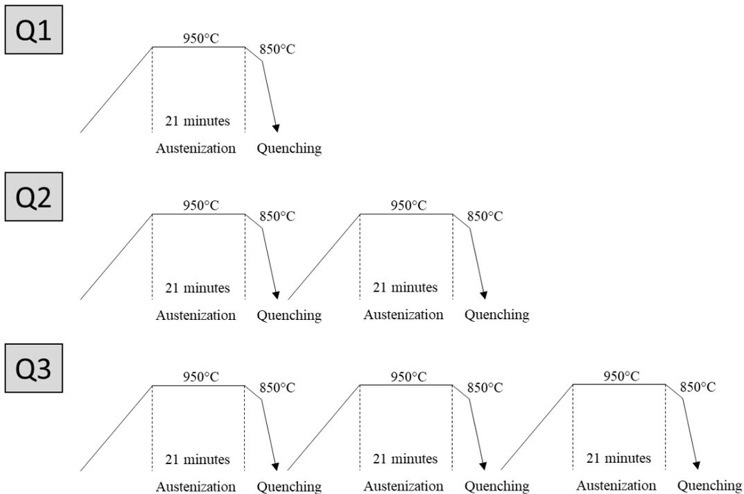
FIGURE 2. Heat Treatment Parameter Cycle for Austenization and Quenching
