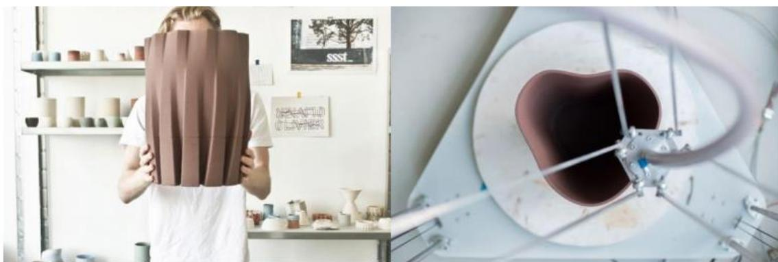
Figure 14. Functional ceramic product made in 3D printing.
